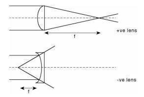
A positive lens forms a real image (an image you can see on a screen) if the object is further than one focal length away from the lens. If the distance from object to lens is u and the distance from lens to image is v, the focus law is
