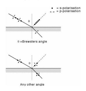
to the surface (p-polarisation), there is a special angle at which all the light goes into the medium and none at all is reflected. This is called Brewster's angle,  $\theta_B$ . It is measured, as always, from the surface normal and is given by the formula
