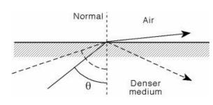
Total internal reflection is part of the explanation of the rainbow, and is used in light guides (optical fibres), "catseyes" (now no longer set in roads) and many optical devices. An important chemical instrument, which you may use in later practicals, is the Abbé refractometer, where total internal reflection is used to determine the refractive indices of liquids with great accuracy.
