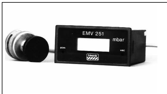
Fig. 2. Diaphragm gauge, set 1 (left). Diaphragm gauge, set 2 (right).
