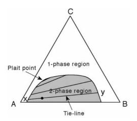
The lengths of the tie-lines gradually diminish as one moves toward corner C. The point at which the tie-line is of negligible length is called the Plait point, and is one of the pieces of data to be found in this experiment.
